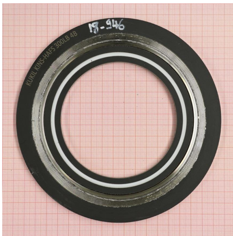
Shell leakage test (T) according MESC SPE 85/300 - 3.3.2
