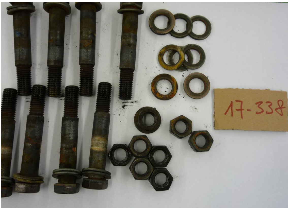
Electrical Isolation kit after the Fire Test (MESC SPE 85/300 - 3.3.15)
