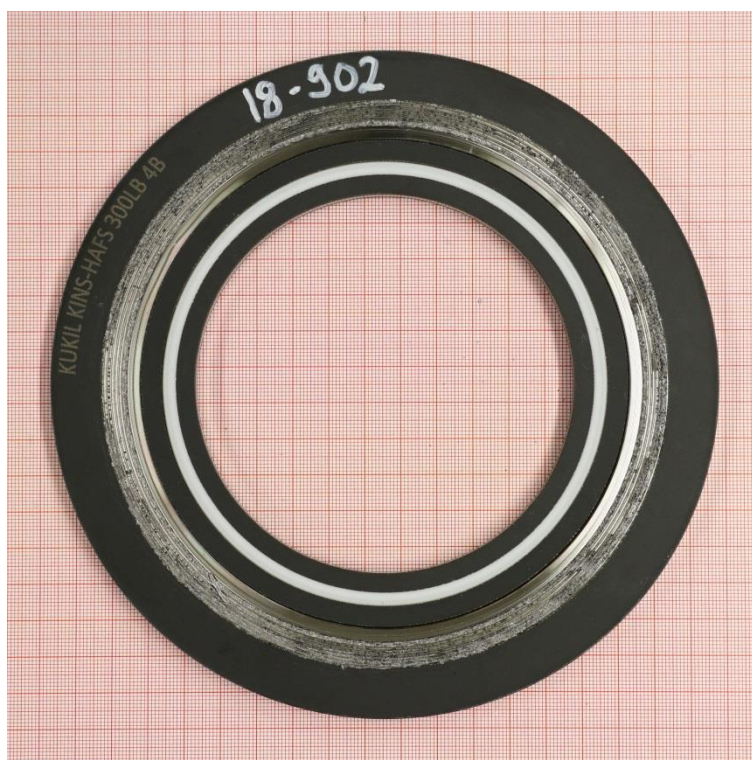
Shell cycle test (T) according MESC SPE 85/300 - 3.3.5
