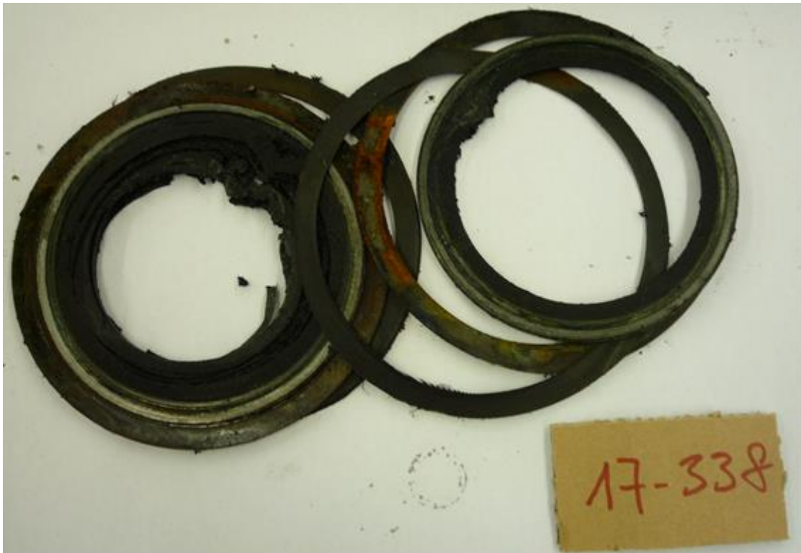
Fire Test according to API 6FB (Shell Specification MESC SPE 85/300 - 3.3.3)
